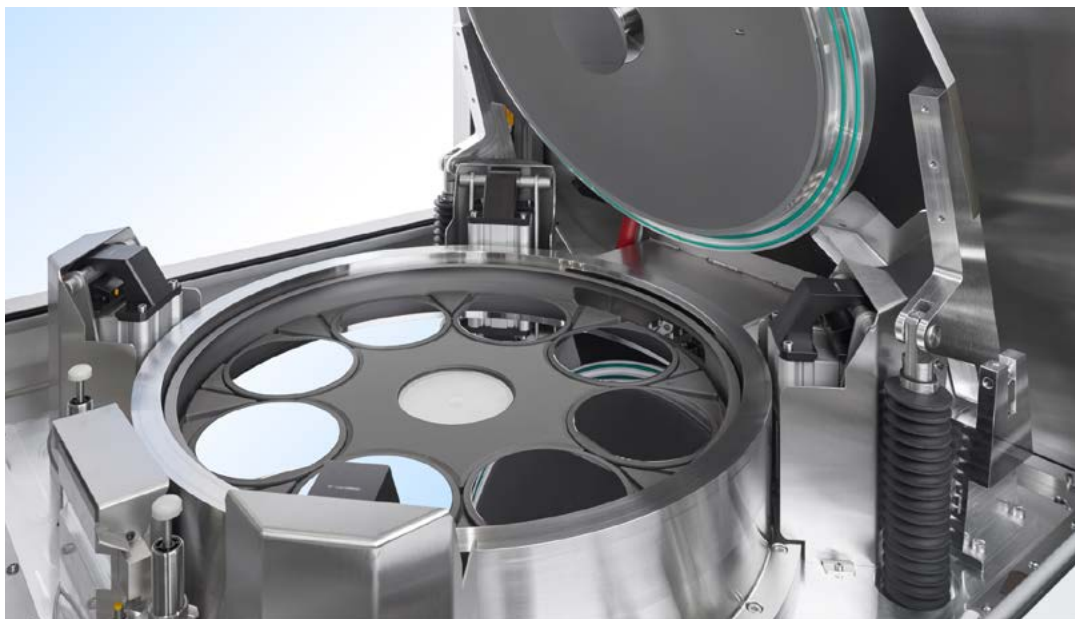
Our tool for laser production: AIX2800G4-TM configuration 8x6 inch.
